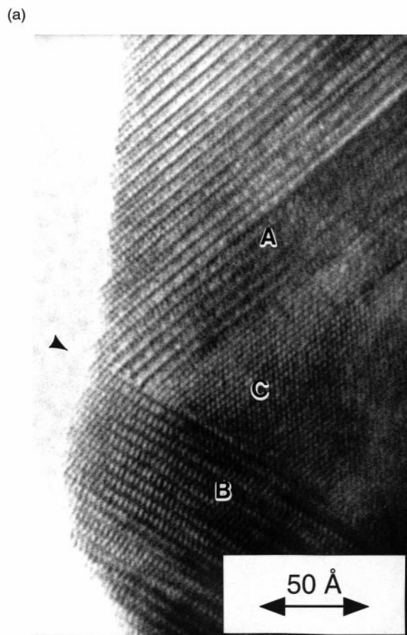
Fig. 4 Electron micrograph of a crystallite with twinning recorded close to the Scherzer focus ( -412 \text{ \AA} ). The arrows on the left denote the twinning planes in the structure. The lattice fringes are tilted by ca. 19^\circ across the twin boundary, as shown by the black-on-white lines.
