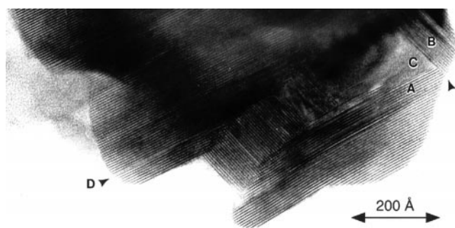
Fig. 7 Electron micrograph showing a group of intergrown crystallites. Regions marked as A, B, and C, and as D, denoted by the arrows in the figure, are magnified in Fig. 8 and 10, respectively.
